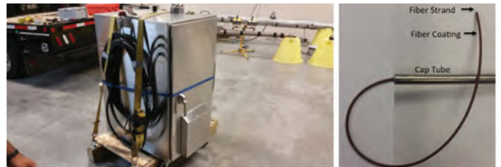
Hifi Enclosure and Fiber Optic Cable
